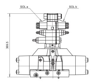
With MT-02W-60 (type W) (Hexagon socket head cap bolts used: M5 x 85, 4 pcs.)
